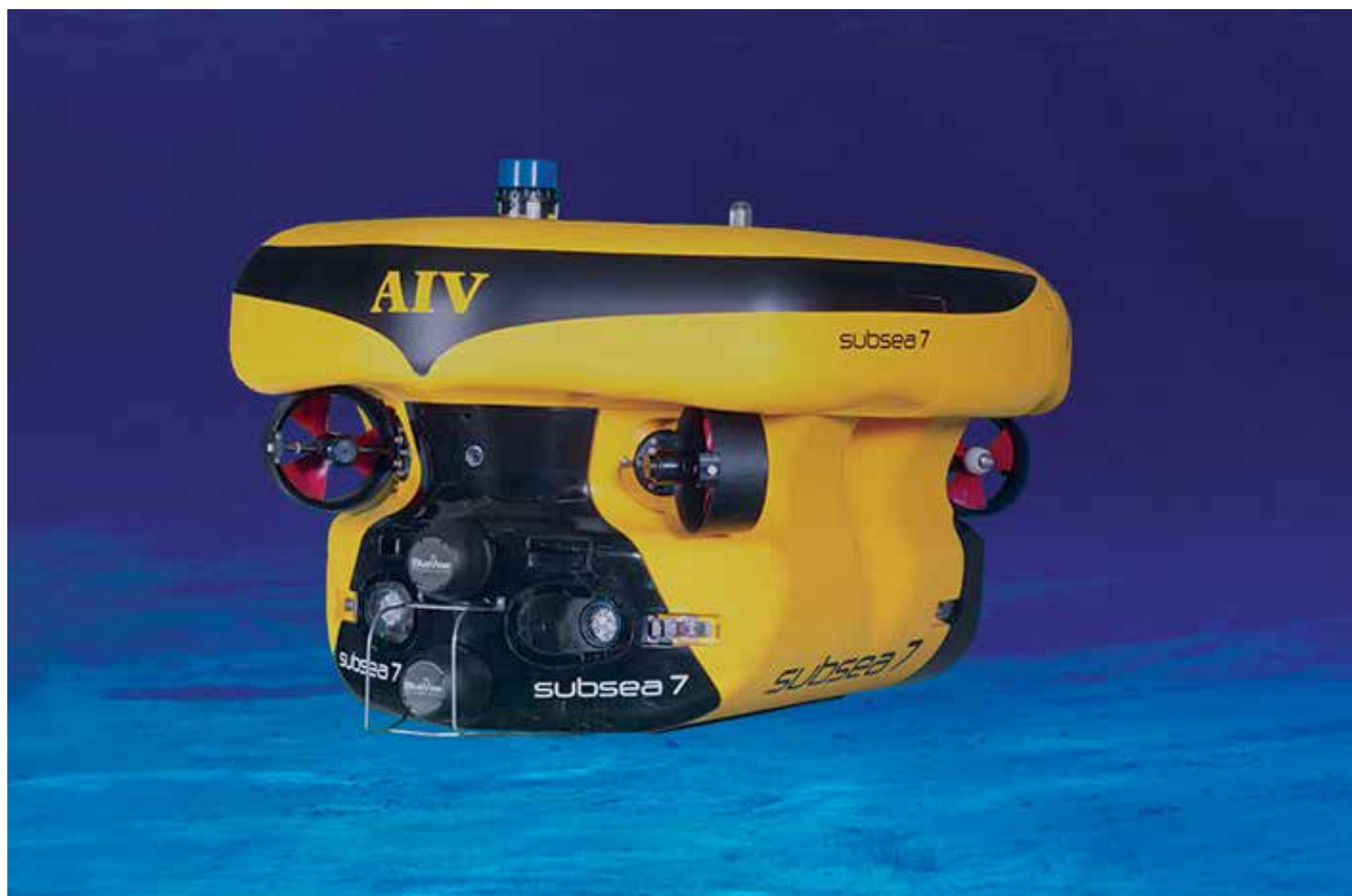
Autonomous inspection vehicle (AIV) – Subsea 7 (Photo: Heriot-Watt University)
